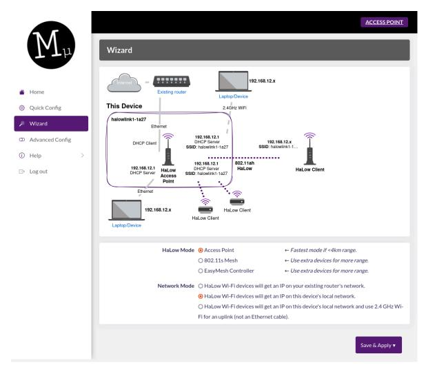
You should see that the option 'HaLow Wi-Fi devices will get an IP on this device's local network' is selected; i.e. this device is acting as a router.
